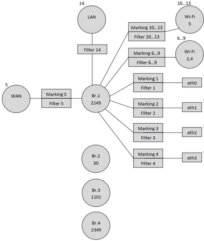
Since it is necessary to configure the receiving of IP address for STB in vlan 2349 behind the ONT eth3 port, it is necessary to bind the bridge of this service (Bridge 4) to the eth3 interface.
