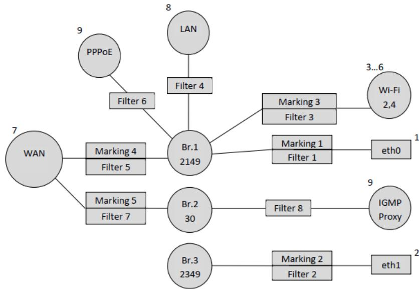
To complete the configuration, bind Bridge 3 to the WAN interface, as we remember, only the filter and marking parameters are required to create the bridge connection:
