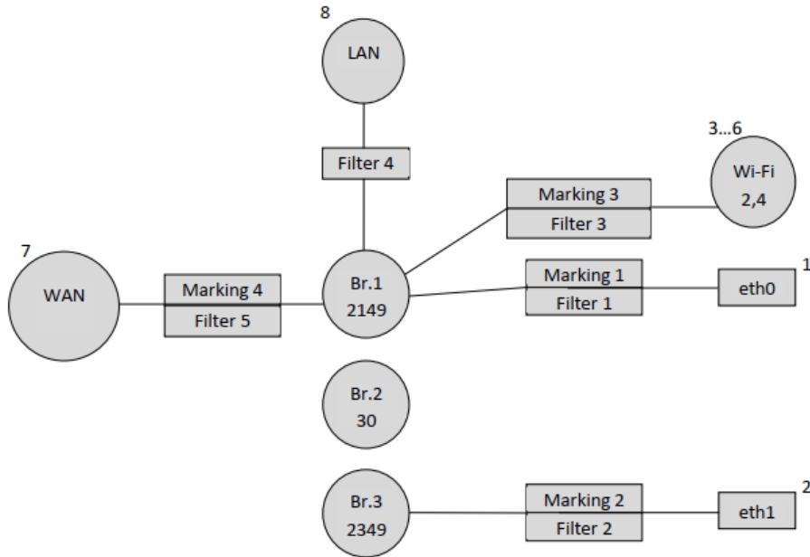
FilterInterface values for interfaces other than the default should be consecutive and start after the highest FilterInterface value in the default configuration. In our case, the highest FilterInterface (interface number) value in the default configuration is 8 (LAN interface). Therefore, FilterInterface for the non-default first interface will be 9.
