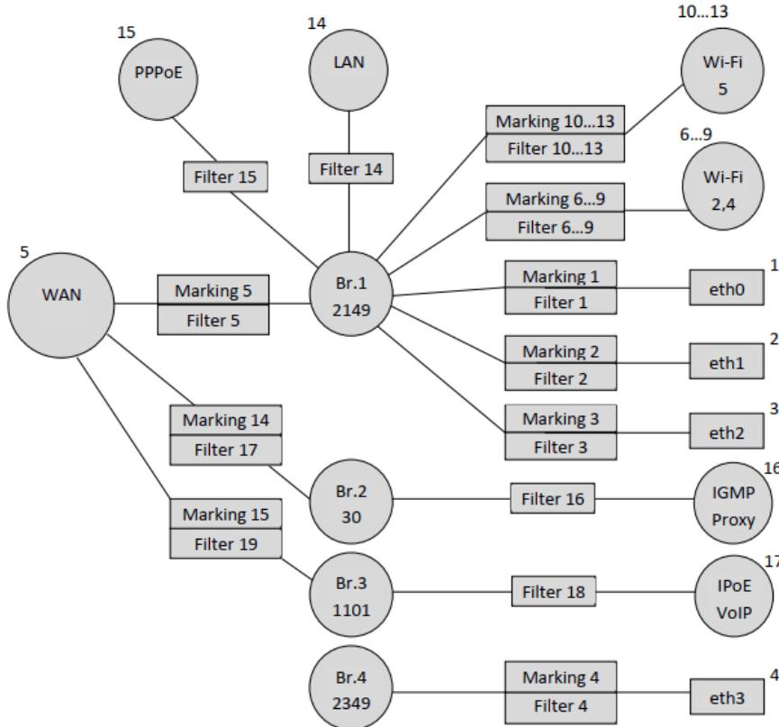
The only thing left is to bind Bridge 4 to the WAN interface using parameters:
