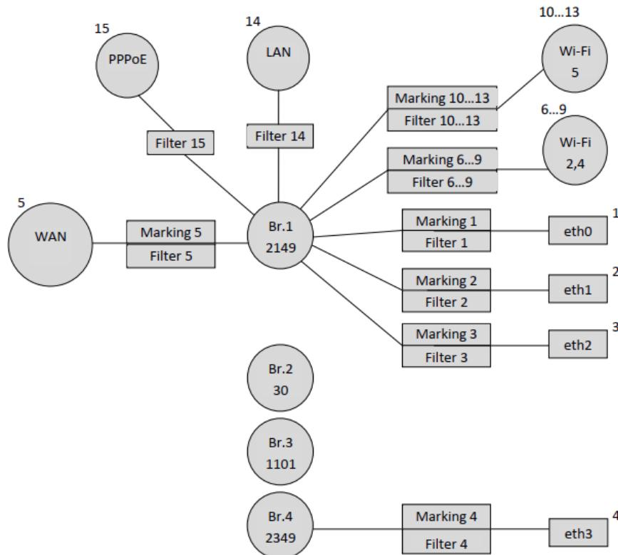
Similarly, we create an IGMP-Proxy interface and bind it to Bridge 2, taking into account that non-default interfaces are bound only by filters.
