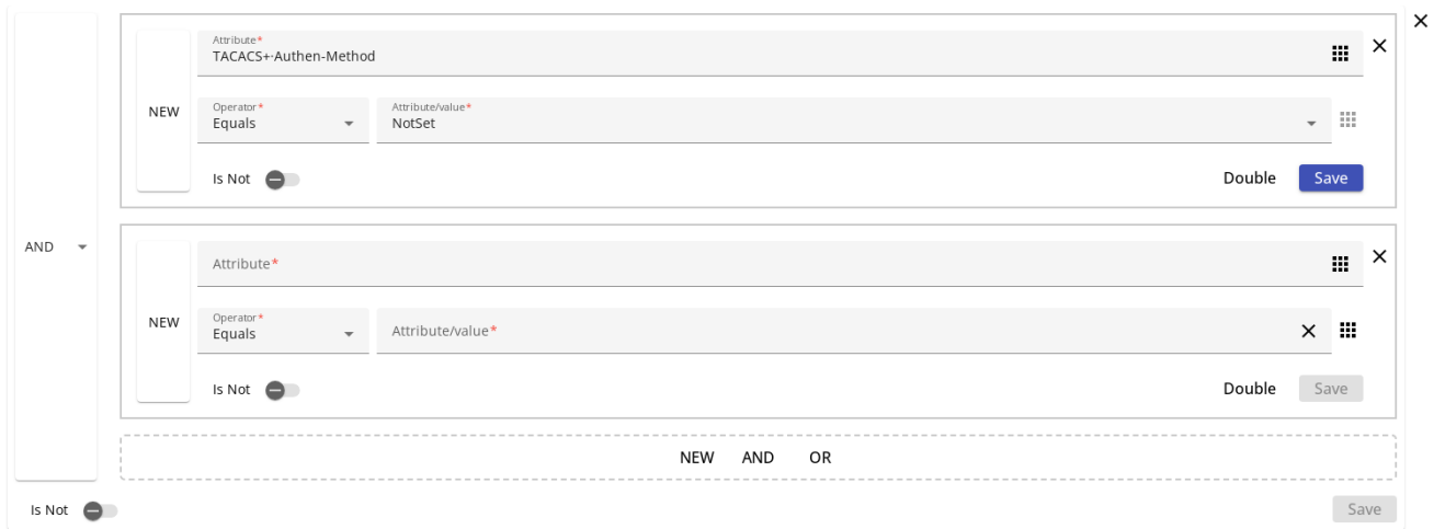
Figure 118. Condition consisting of two conditions combined by a logical "AND"
