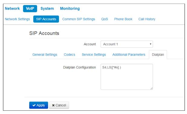
To define a dialplan, use regular expressions in the 'Dial plan configuration' field. The structure and format of regular expressions that enable different dialling features are listed below.
