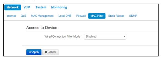
Wired Connection Filter Mode — define one of the three filter operation modes depending on the host's MAC address:
