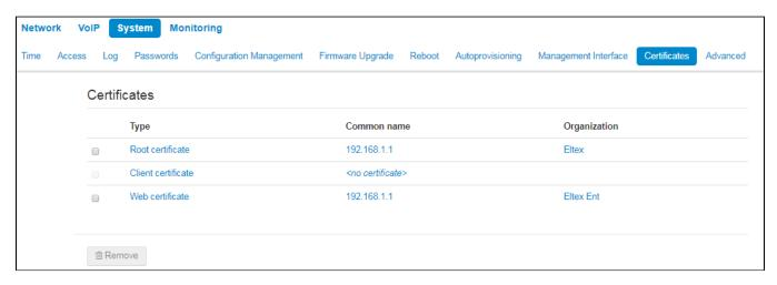
'Certificates' submenu allows to view, download and upload certificates for using in protected TLS connections.
