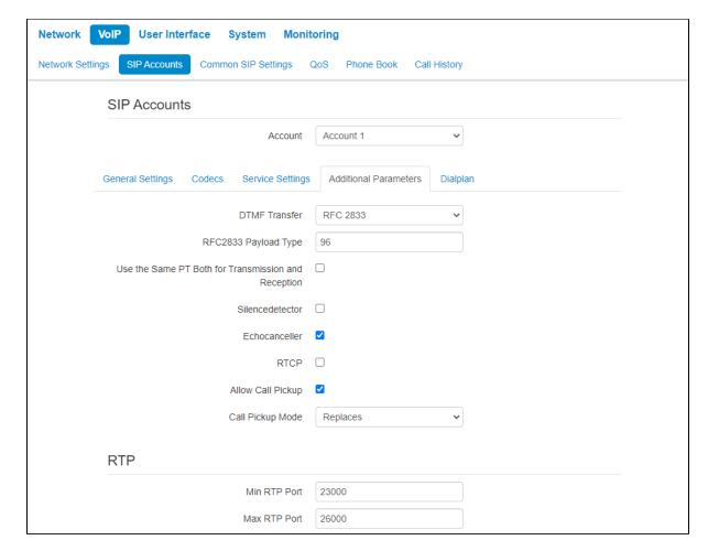
*DTMF Transfer* — mode of DTMF signal transmission:
