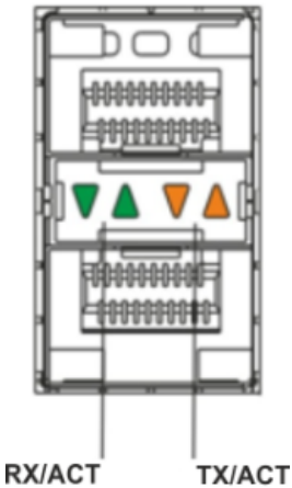
Figure 39 – Location of optical interface indicators
