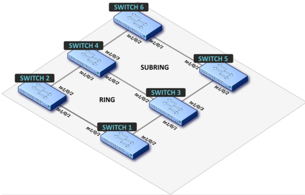
, . ERPS VLAN 10 (R-APS VLAN), VLAN 20, 30, 40, 200, 300, 400. ERPS VLAN 100, VLAN 200, 300, 400. , , (1 2), VLAN .
